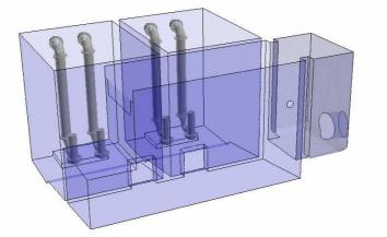
In the recent scheme shown below, pre-swirl levels were found to exceed design standards and excessive operational pump wear was predicted. By making (relatively minor) changes to the design the lifetime of a  $\pm 1.2$ m pumping station was significantly extended.
